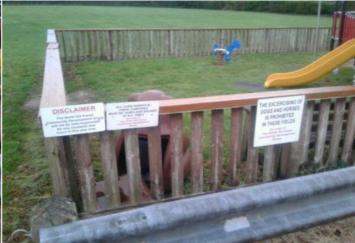
**Finding:** BS EN 1176 Part 7 recommends that signage shall **Action**: Provide additional information include emergency contact details and contact details of owner / operator for reporting maintenance issues
